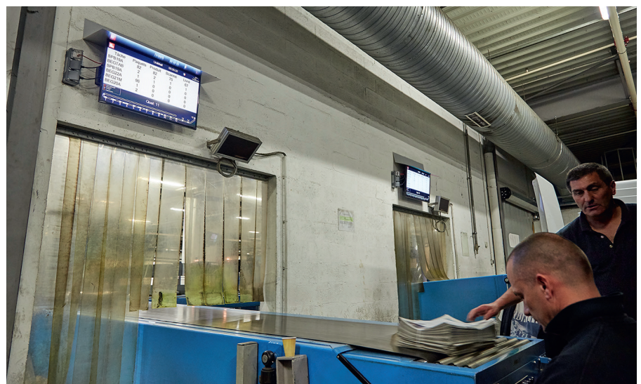
One monitor at each loading dock provides the driver with detailed information about the current route, the number of bundles already and still to be produced, plus the bundles that have reached the loading dock.
